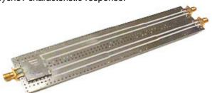
The unbalanced port return loss plot was measured at the input of the aforementioned test board. Unbalanced port return loss performance can be improved as narrow band matching is performed at the output of the balun (input of the transistor).
